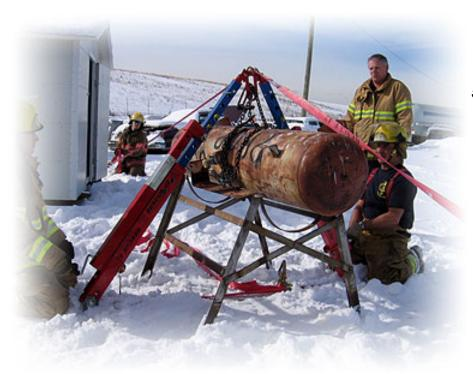
5,000 lb working load 10.000 lb test load
