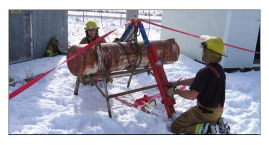
automatically pivot so that the tongue is pointed in the direction of the load. You may also use the A-frame sideways (try using Spike Feet) to pull car doors or metal outwards.
