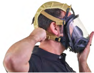
Figure 3-8 Tightening the neck straps
