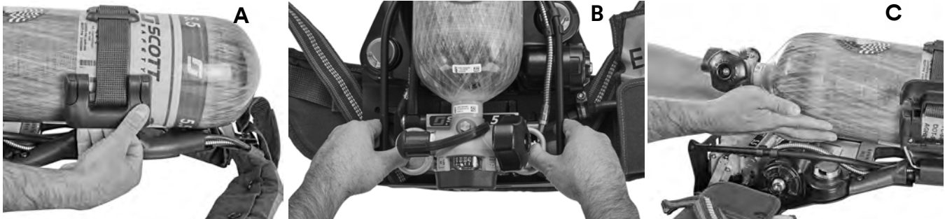
Figure 3-17 A) Disengaging the cylinder retention latch plate. B) Pulling the Snap-Change locks horizontally away from the pressure reducer. C) Lifting the cylinder free from the backframe.
