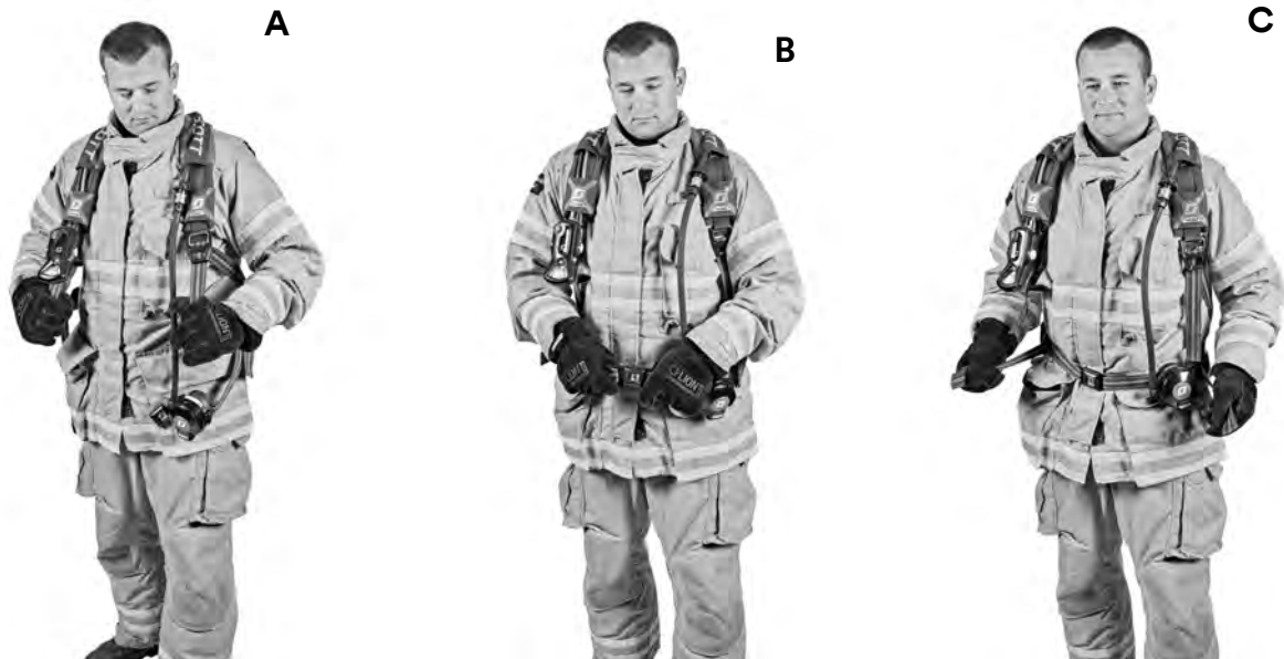
Figure 3-2 A) Pulling the shoulder straps down. B) Connecting the waist pad buckle. C) Adjusting the shoulder pads.
