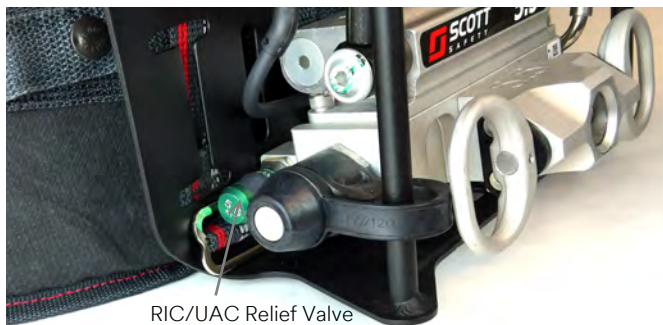
Figure 2-2 Inspecting the RIC/UAC connection
