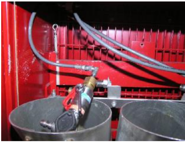
New method of positioning hose with right angle elbow pointed to the left..
