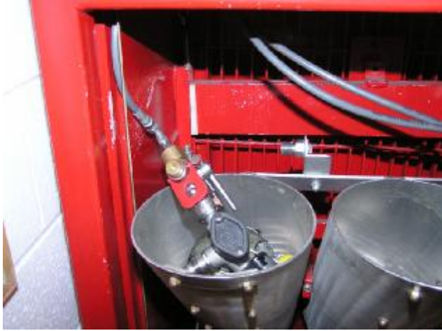
The old method of positioning hose. Note metal on metal rubbing with right angle elbow pointed up.
